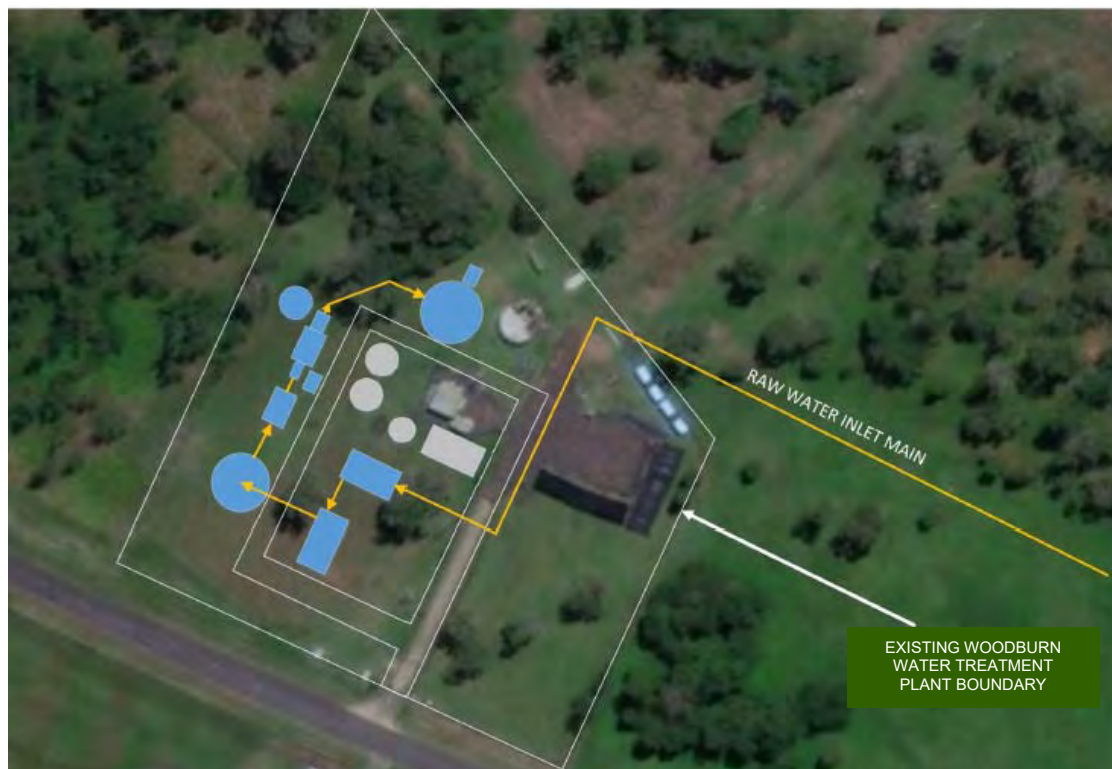
Figure 12: Woodburn groundwater WTP inlet and layout
